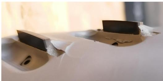
Figure 2 – Aluminium milling tool prototype after EDM sharpening.
