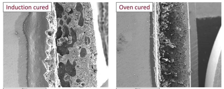
Figure 5 – Scanning electron micrograph of the fractured surfaces of induction cured and oven cured specimens
