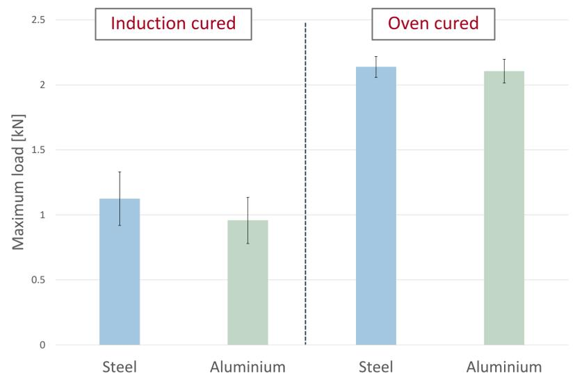
Figure 4 – Maximum shear load [kN] for induction cured and oven cured steel and aluminium specimens.
